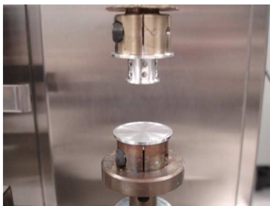
Figure 2. Upper and lower portions of rheology fixtures used to measure viscosity of flashing and curing clearcoats. The "well" in the lower platen retains \sim 50 \mu\text{m} of clearcoat. Oscillation occurs about the hollow vertical axis of the upper fixture.
